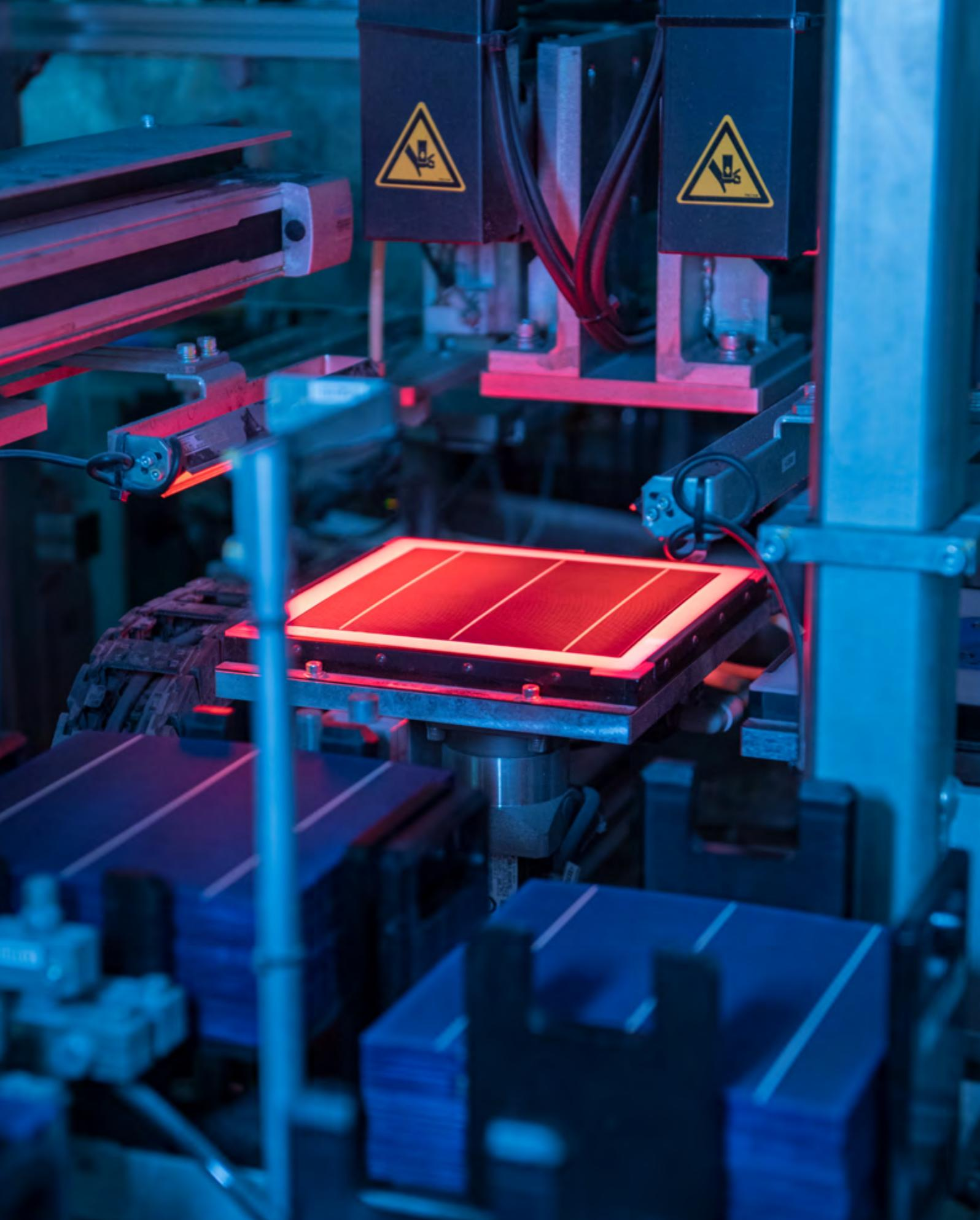
WINAICO attaches great importance to non-contact production processes. The busbars are soldered in a high-precision process to what are known as strings. Highly reflective strips are then attached to the front and back of the cells.
